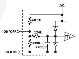
Figure B: Internal ON/OFF pin circuitry
