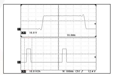
Figure 18: Load current (10A/div) as a function of time (10ms/div and 100ms/ div) when the converter attempts to turn on into a 10 m $\Omega$  short circuit.
