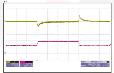
Figure 11: Output voltage response to step-change in load current (50%-75%-50% of lout(max); dI/dt = 0.1 A/µs). Load cap: 1µF ceramic and 15µF tantalum capacitors. Ch 1: Vout (500mV/div), Ch 2: lout (10A/div). Timescale: 500µs/div.
