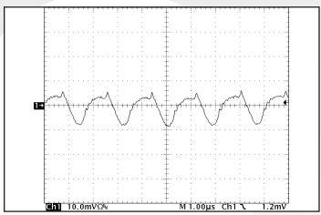
Figure 9: Input terminal current ripple,  $i_C$ , at full rated output current and nominal input voltage with  $100\mu H$  source impedance and  $47\mu F$  electrolytic capacitor 100mA/div). Bandwidth: 20MHz. Timescale:  $1.00\mu s/div$ . See Figure
