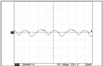
**Figure 10:** Output voltage ripple, Vout, at nominal input voltage and rated load current (200 mV/div). Load capacitance: 1μF ceramic capacitor and 15μF tantalum capacitor. Bandwidth: 10 MHz. Timescale: 1.00μs/div. See Figure 17.
